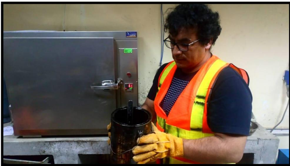
Figura 22: 30 gr. De Asfalto a  $140 \pm 5 \text{ C}^\circ$
