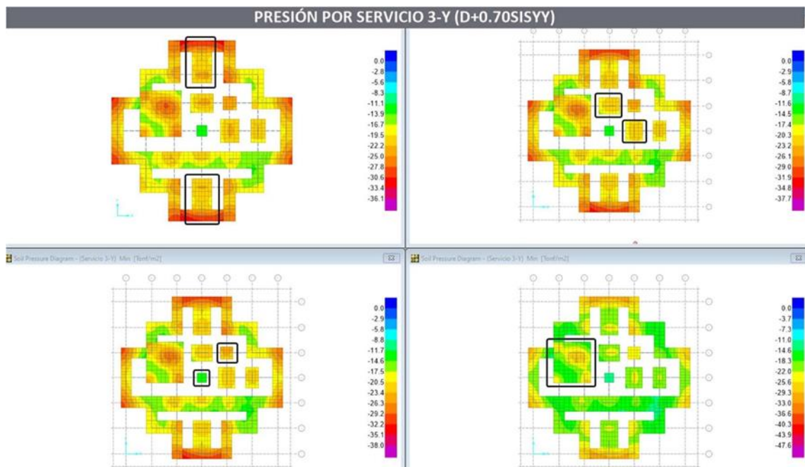
Figura 83 – Presión – Servicio 3-Y (D+0.70SY) / Qadm = [27.10, 28.30, 28.50, 35.70]*4/3 Tonf/m2.
