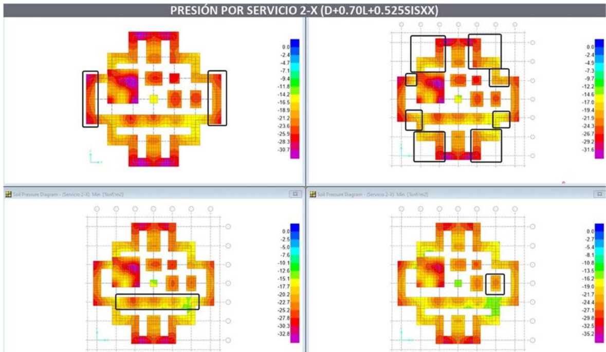
Figura 76 – Presión – Servicio 2-X (D+0.70L+0.525SX) / Qadm = [23.00, 23.70, 24.60, 26.40]*4/3 Tonf/m2.
