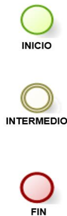
Figura Nro. 2.3.5 Tipos de eventos del flujo Business Process Model and Notation (BPMN)
