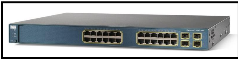
Fig. 20: Switch Cisco Catalys 3560 de 12 puertos
