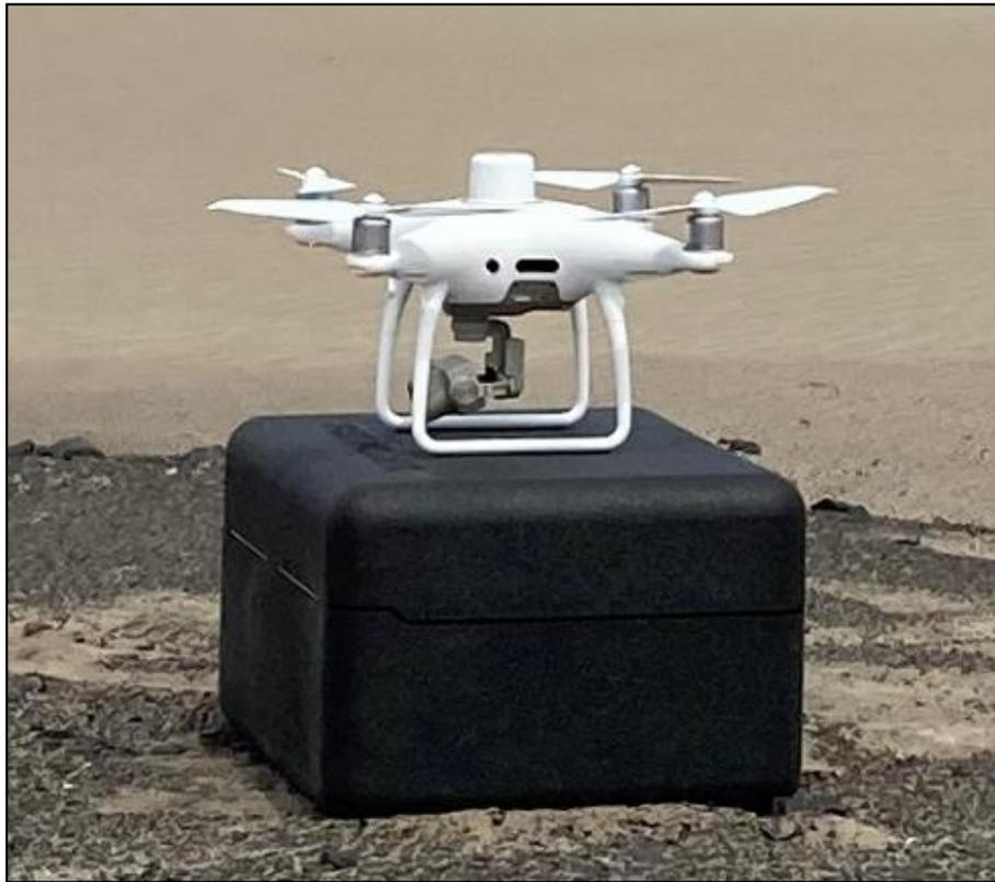
**Figura 11** Phantom 4 RTK
