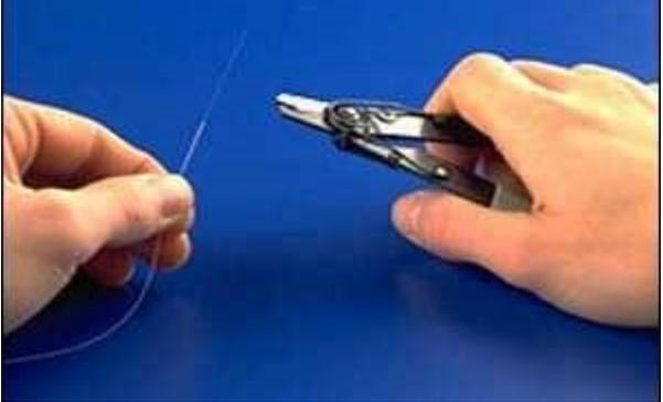
A close-up photograph showing a person's hands using a pair of special tweezers to strip the outer coating of an optical fiber. The fiber is held taut, and the tweezers are positioned to peel away a section of the coating. The background is a solid blue color.                |
