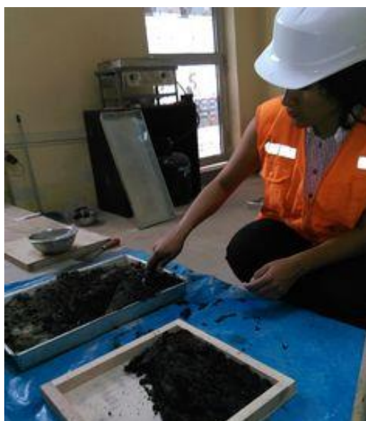
Figura 34: Molde de Slurry Seal
