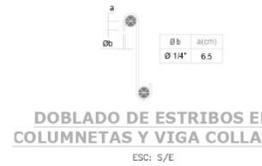
**DOBLADO DE ESTRIBOS EN COLUMNETAS Y VIGA COLLARIN**
