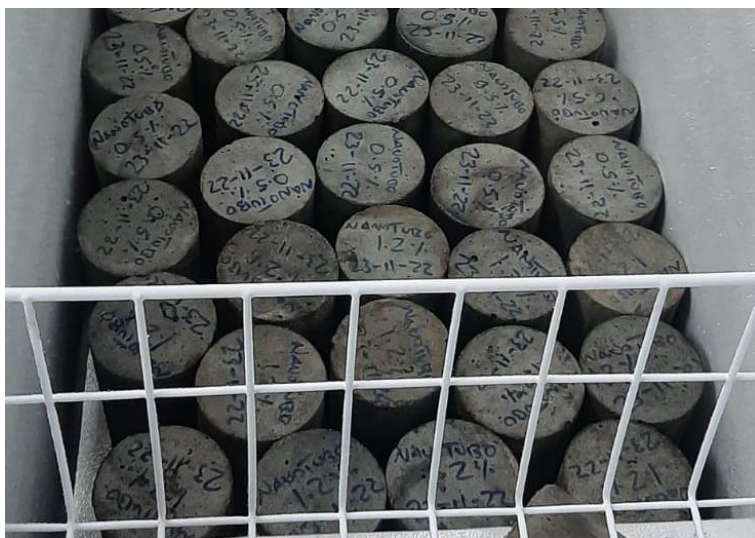
Figura 5.23 Probetas a temperaturas de -8^{\circ}\text{C} a -10^{\circ}\text{C} .
